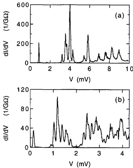
Fig. 3. Differential conductance at 30mK for two very small particles, showing the spectrum of eigenstate energies. For (a),  $C_1 = 1.5$  aF,  $C_2 = 3.2$  aF, particle volume  $\approx 40$  nm<sup>3</sup>, for (b),  $C_1 = 2.5$  aF,  $C_2 = 6.3$  aF, particle volume  $\approx 100$  nm<sup>3</sup>.
