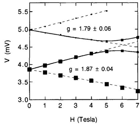
Fig. 4. Bias position of peaks in  $dI/dV$ , plotted versus magnetic field, showing the evolution of eigenstate energies with  $H$ . To convert from voltage to eigenstate spacing, multiply by  $eC_1/(C_1 + C_2) = 0.54$  meV/mV. Area of symbols represents the magnitude of current carried by each state. Dotted lines: extrapolation of linear Zeeman splitting at low fields. Solid lines: solution of  $2 \times 2$  matrix Hamiltonian with spin-orbit matrix element of  $77 \mu\text{eV}$ .
