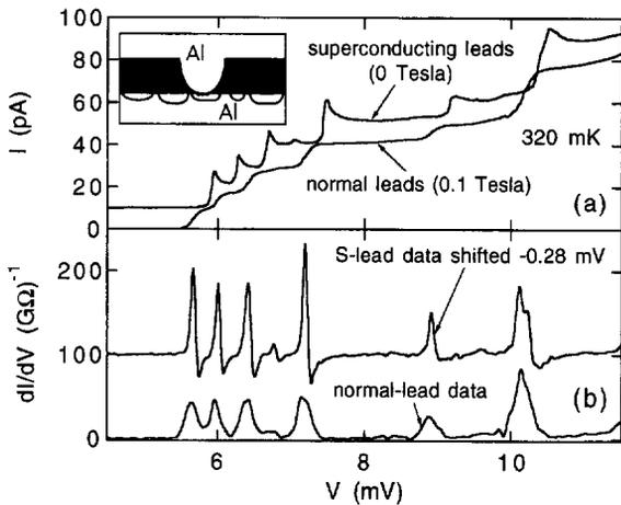
Fig. 1. (a) Current steps due to tunneling via discrete eigenstates on an Al particle. (b)  $dI/dV$  versus  $V$  for the same sample. Data for superconducting leads are offset in  $I$  or  $dI/dV$  for visibility. For this particle, we determine from the Coulomb staircase that  $C_1 = 4.7$  aF,  $C_2 = 8.3$  aF, so particle volume  $\approx 150$  nm<sup>3</sup>. Inset: schematic diagram of device.
