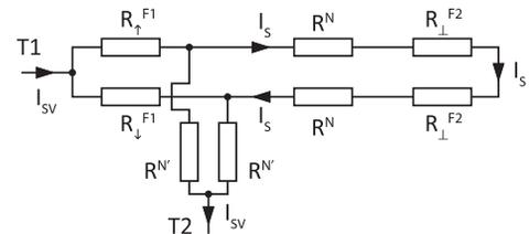
FIG. 3. Effective circuit for modeling spin currents when  $\theta_{SV} = 90^\circ$ . The total current of spin angular momentum absorbed by layer F2 is  $2(\hbar/2e)I_S$ .
