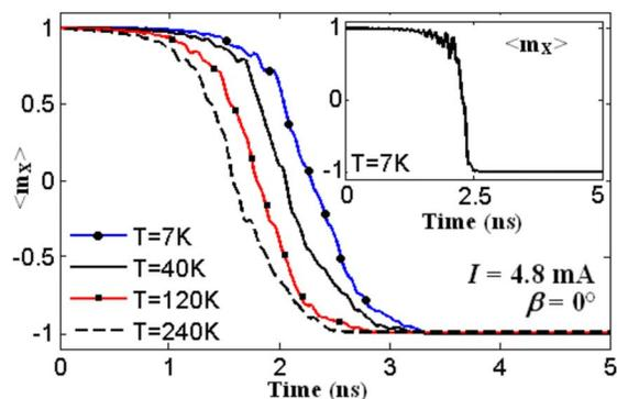
FIG. 6. (Color online) Temporal evolution of the  $x$  component of the magnetization for LR  $\rightarrow$  HR reversal for  $\beta=0^\circ$  at four background temperatures (7, 40, 120, and 240 K), averaged over 50 iterations. Inset: temporal evolution of the  $x$  component of the magnetization for a single iteration of a LR  $\rightarrow$  HR reversal for a background temperature of 7 K.
