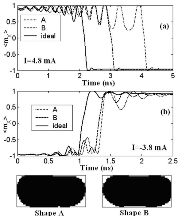
FIG. 3. Temporal evolution of the  $x$  component of magnetization for an ideal ellipse and two nonideal shapes (A and B) for  $\beta=30^\circ$ . (a) LR  $\rightarrow$  HR switching; center: (b) HR  $\rightarrow$  LR switching. Bottom: the nonideal shapes used for performing our simulations.
