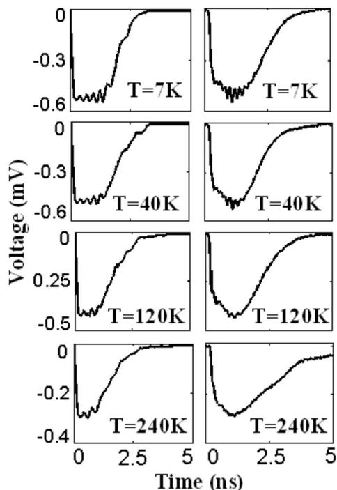
FIG. 4. A comparison between computed (left) and experimentally measured (right) voltage signals due to current-induced magnetization reversal from the low- to the high-resistance state for  $\beta=30^\circ$  at four background temperatures (7, 40, 120, and 240 K) and a current of 4.8 mA.
