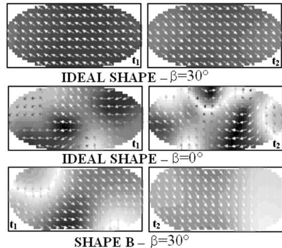
FIG. 2. Snapshots of the magnetization configuration during the reversal processes shown in Figs. 1 and 3. Top: ideal shape with  $\beta=30^\circ$  at  $t_1=0.93$  ns and  $t_2=1.35$  ns. Center: ideal shape with  $\beta=0^\circ$  at  $t_1=5.27$  ns and  $t_2=6$  ns. Bottom: shape B (see Fig. 3) with  $\beta=30^\circ$  at  $t_1=1.38$  ns and  $t_2=1.67$  ns.
