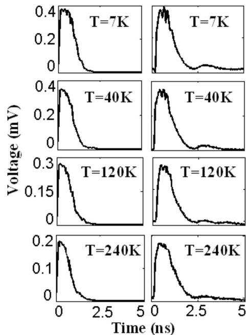
FIG. 5. A comparison between computed (left) and experimentally measured (right) voltage signals due to current-induced magnetization reversal from the high to the low resistance state for  $\beta=30^\circ$  at four background temperatures (7, 40, 120, and 240 K) with a current of  $-3.8$  mA.
