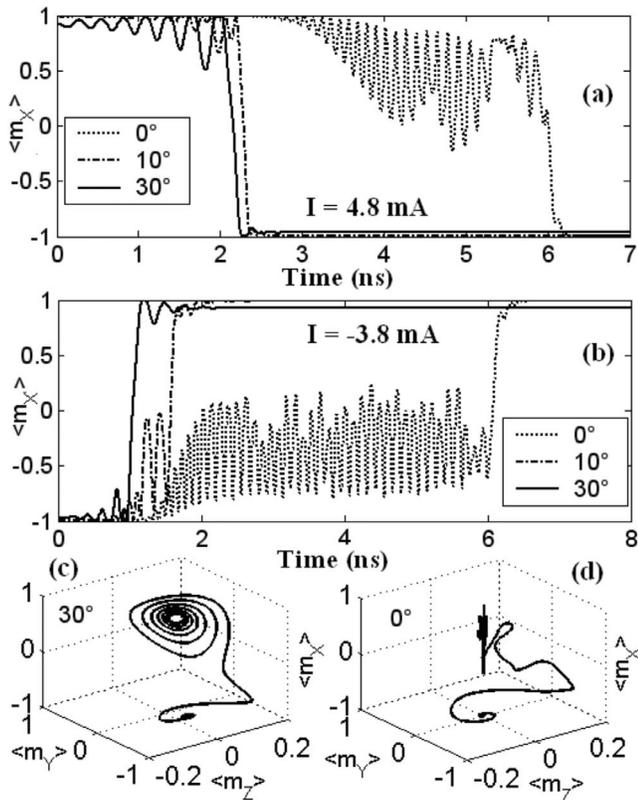
FIG. 1. Temporal evolution of the  $x$  component of the magnetization for three initial offset angles between the pinned and free magnetic layers ( $\beta=0^\circ$ ,  $10^\circ$ , and  $30^\circ$ ). (a) LR→HR reversal; (b) HR→LR switching. Bottom: trajectories of the average magnetization during LR→HR reversal for (c)  $\beta=30^\circ$  and (d)  $\beta=0^\circ$ .
