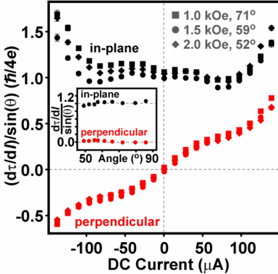
Supplementary Figure S4. Values of the in-plane and out-of plane differential torques  $d\tau_{\parallel}/dI$  (black symbols) and  $d\tau_{\perp}/dI$  (red symbols) vs.  $I$ , determined from fits to room-temperature ST-FMR spectra. The overall scale for the y-axis has an uncertainty of  $\sim 15\%$  associated with the determination of the sample volume. (Inset) Angular dependence of the differential torques at zero bias.
