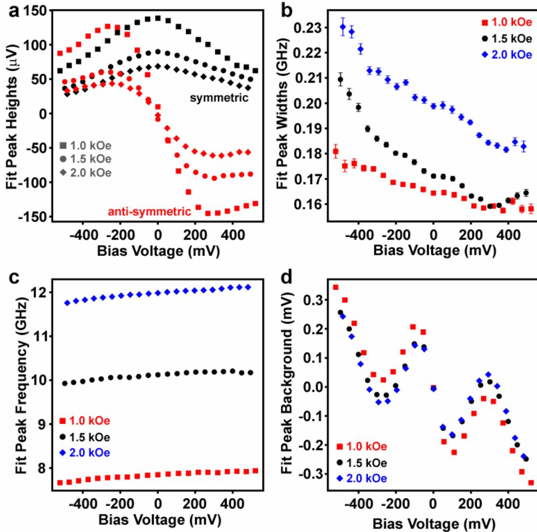
Supplementary Figure S1. Fit parameters for the ST-FMR signals at room temperature, for three values of magnetic field in the  $\hat{z}$  direction and  $I_{RF} \approx 12 \mu\text{A}$ . (a) Amplitudes of the symmetric and antisymmetric Lorentzian component of each peak. (b) The linewidths  $\sigma/(2\pi)$ . (c) The center frequencies  $\omega/(2\pi)$ . (d) Non-resonant background components.
