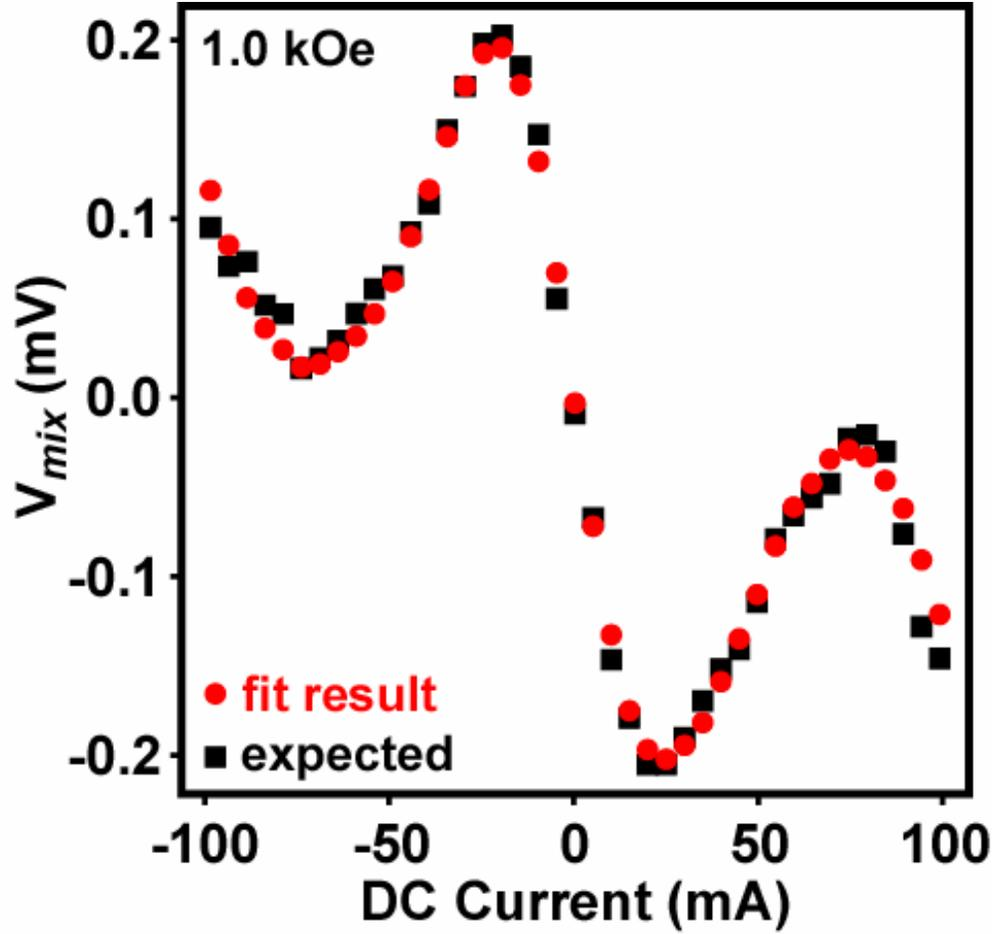
Supplementary Figure S2. Test of the calibration for  $I_{RF}$  and the non-resonant background, for  $H = 1.0$  kOe in the  $\hat{z}$  direction. Circles: Magnitude of non-resonant background measured from fits to the ST-FMR peaks. Squares: the background expected from Equations (S9) and (S10) after determining  $I_{RF} = 11.7 \mu\text{A}$  at  $I_0 = -30 \mu\text{A}$ .
