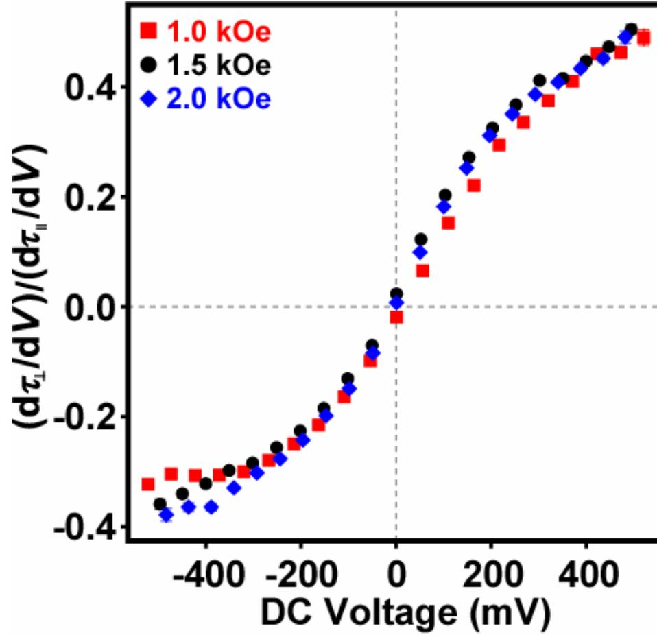
Supplementary Figure S5. Ratio of the perpendicular torkance  $d\tau_{\perp}/dV$  to the in-plane torkance  $d\tau_{\parallel}/dV$  as a function of bias.
