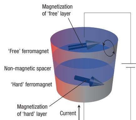
**Figure 1** Excitation of a ferromagnet by spin-transfer torque. The passage of a current through a 'hard' magnetic layer causes it to become spin-polarized. When this current is subsequently injected across a thin non-magnetic spacer layer and into a 'free' magnetic layer, the realignment of its polarization induces a torque on the magnetic moment of the free layer, causing it to precess and even reverse.
