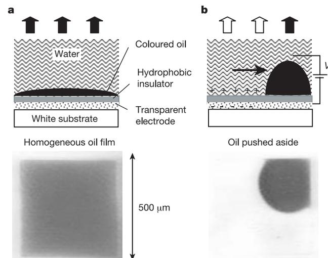
**Figure 1** Electrowetting display principle. **a**, No voltage applied, therefore a coloured homogeneous oil film is present. **b**, d.c. voltage applied, causing the oil film to contract. Top row, diagrams; bottom row, photographs. The photographs show typical oil motion obtained with an homogeneous pixel electrode.
