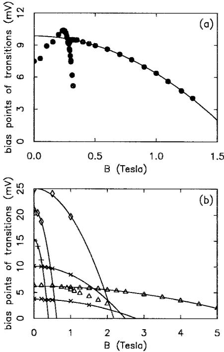
Fig. 12. (a) Transition voltage  $V_c(H)$  of the conductance transition [32] as a function of magnetic field for a quenched Cu constriction at 4.2 K, showing bifurcation (Cu.9b, iv). At high fields  $V_c(H) \rightarrow 0$  (Cu.9b, v), the dependence on  $H$  being quadratic. (b)  $V_c(H)$  for five other samples at 4.2 K, with associated decreases to 0, quadratically in  $H$ .
