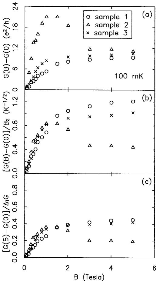
Fig. 14. Magnetic field dependence of the  $V=0$  conductance for the 3 unannealed Cu samples at 100 mK. (a) Absolute magnetoconductance. (b) Magnetoconductance scaled by the value of  $B_z$  for each sample. (c) Magnetoconductance relative to the change in conductance between 100 mK and 6 K. An applied magnetic field alters, but does not eliminate, the zero-bias conductance signal due to TLSs.
