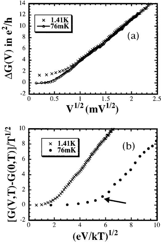
Fig. 16. (a)  $\Delta G(V) = G(V, T) - G(0, 0.76 \text{ mK})$  vs.  $V^{1/2}$  for a  $19\Omega$  Ti construction (sample 5) at 1.41 K and 76 mK. (b) The same data do *not* scale when plotted as  $[G(V, T) - G(0, T)]/T^{1/2}$  vs.  $(eV/k_B T)^{1/2}$ , due to “premature saturation” (see arrow) of the 76 mK curve, as discussed in (Ti.3).
