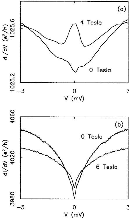
Fig. 4. (a) Conductance signals for 500 ppm magnetic Mn impurities in Cu at 100 mK, showing Zeeman splitting in an applied magnetic field. (b) The ZBA signals from quenched Cu samples exhibit no Zeeman splitting, demonstrating that they are not due to a magnetic impurity. However, the shape and amplitude of the ZBA does depend on magnetic field.
