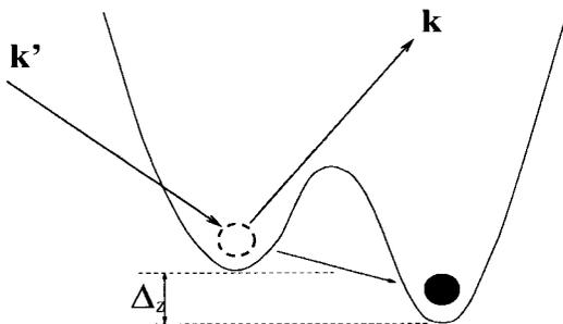
Fig. 6. A generic two-level-system, with (bare) energy asymmetry  $\Delta_z$  and tunneling rate  $\Delta_x$ . An electron-assisted tunneling event is depicted: an electron scatters of the TLS and induces the atom to tunnel.
