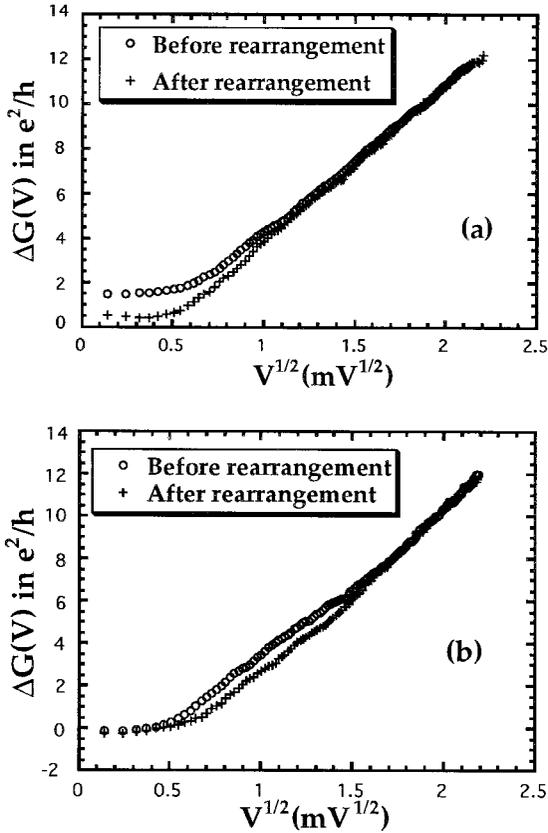
Fig. 17. (a) The ZBA of the Ti sample 5 before and after electromigration [see (Ti.4)], which changed the saturation energy  $T_x$  of Eq. (29) from 2.3 to 1.4 K. (b) A  $22\Omega$  Ti constriction (sample 6) shows two distinct saturation energies  $T_{x1}$  and  $T_{x2}$ , which change upon electromigration from 0.9 to 1.5 K and 9.7 to 6.8 K, respectively.
