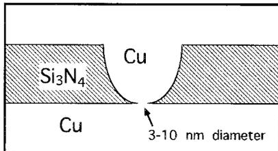
Fig. 1. Cross-sectional schematic of a metal nanoconstriction. The hole at the lower edge of the  $\text{Si}_3\text{N}_4$  is so small that this region completely dominates the resistance of the device.
