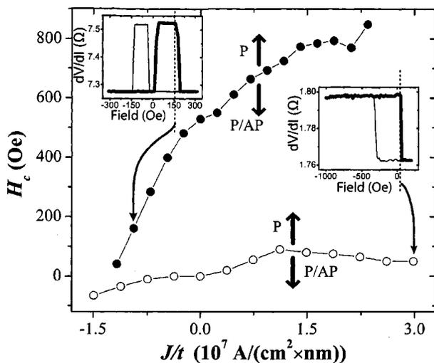
FIG. 3.  $H_c$  plotted vs  $J/t$ , the current density normalized to the  $\text{Co}_{\text{free}}$  layer thickness, for normal ( $\bullet$ ) and SAF ( $\circ$ ) samples. The data illustrate the boundary separating the bistable P/AP region and the stable P region as shown. Insets show how  $H_c$  was measured.
