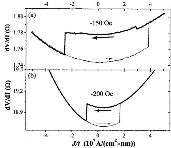
FIG. 2.  $dV/dI$  vs current density normalized to the free layer thickness  $J/t$  for (a) a  $90 \times 190 \text{ nm}$  elliptical SAF sample and (b) a  $70 \times 130 \text{ nm}$  elliptical normal sample. The resistance values in (b), a two-point measurement, include lead resistance  $\sim 6 \Omega$  and contact resistance  $\sim 9 \Omega$ .
