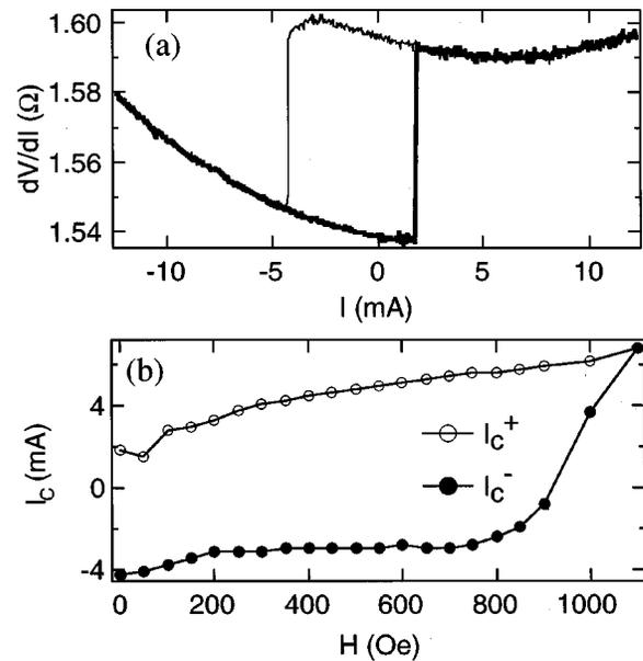
FIG. 2. (a)  $dV/dI$  of a nanopillar spin-transfer device as a function of the applied current through the device. The current is defined as positive when the spin-polarized electrons are flowing from the nanomagnet to the thick Co film. (b) The critical currents  $I_c^+$  and  $I_c^-$  that switch the nanomagnet into, respectively, antiparallel and parallel alignment with the Co film as a function of  $H$ . This data was taken with  $H$  increasing from zero to its maximum value of 1100 Oe.
