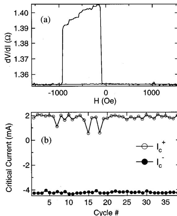
FIG. 3. (a) An example of the magnetoresistance behavior of a nanopillar device for a field cycle in which the nanomagnet switches at the same point that the thick Co film switches, presumably due to domain wall coupling. (b) The critical currents for spin-transfer switching for 30 cycles of the applied current to  $\pm 5 \text{ mA}$ .
